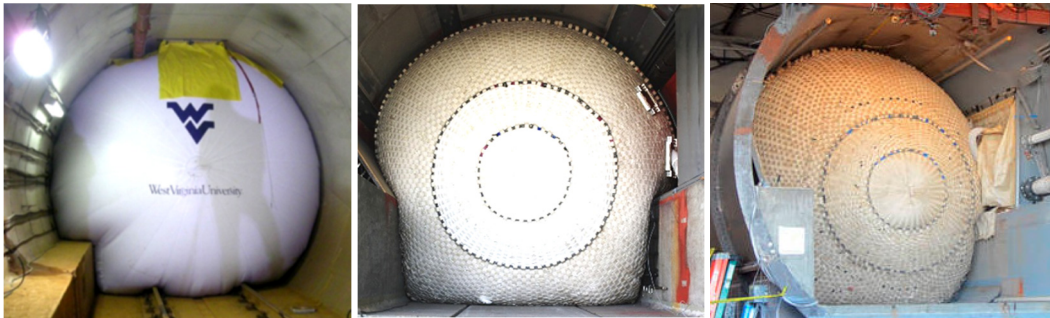
Figure 1: Full-Scale Inflatable Plugs: a) Test performed in an actual tunnel in 2008 (Barrie, 2008, Martinez et al, 2012); b) and c) Tests performed at WVU (Barbero et al, 2013-a, Sosa et al, 2014-a/b).
