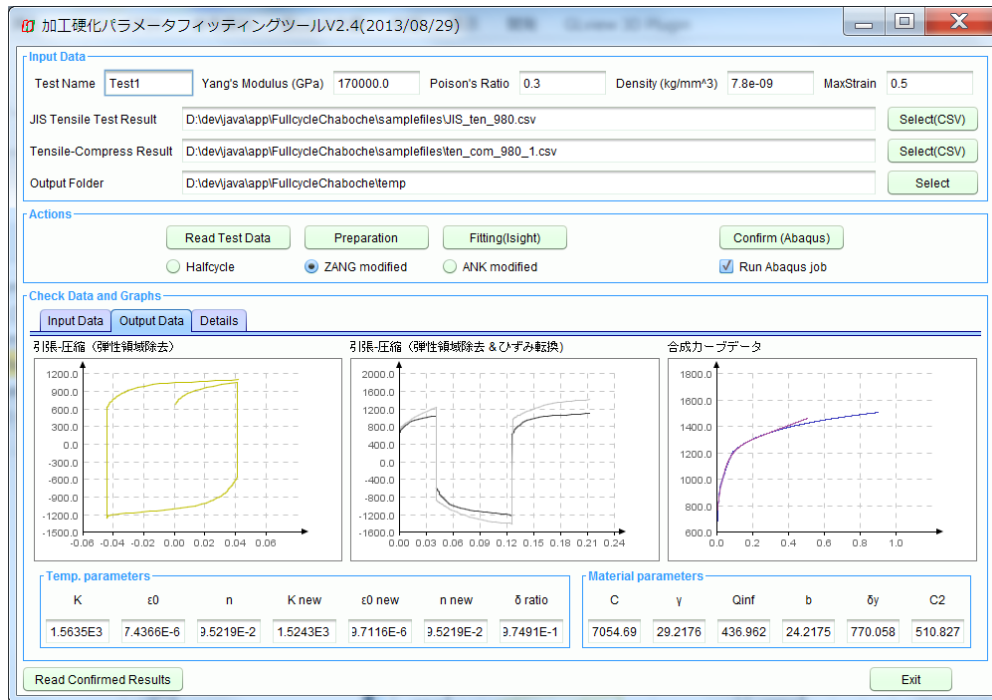
Figure 10. A Java program for fitting material parameters of Chaboche models
