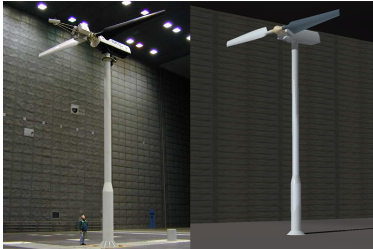
Figure 1: Left: Original wind turbine in the NASA Ames wind tunnel (Hand, 2001). Right: CATIA CAD model (Sicklinger, 2014b).
