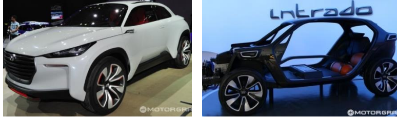
Figure 2. Intrado Full car & BIW with chassis
