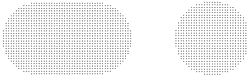
Figure 17 4lb SPH bird model
