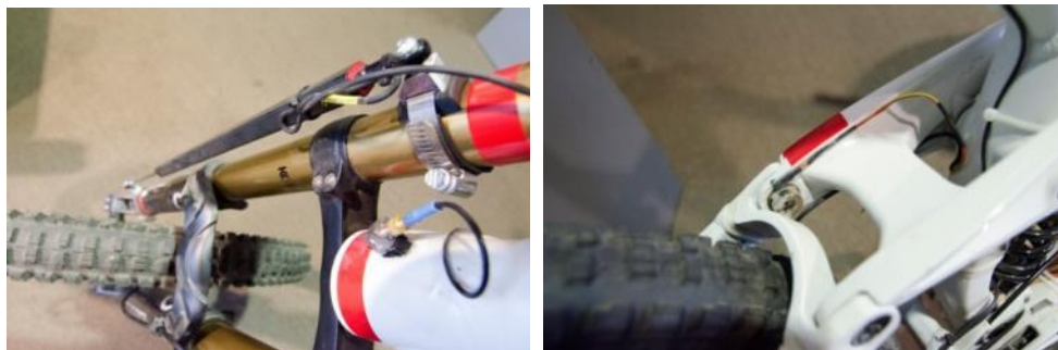
Figure 6. Linear potentiometer (left) used for front fork displacement measurements and Hall Effect sensor (right) used for rear shock displacement measurements.
