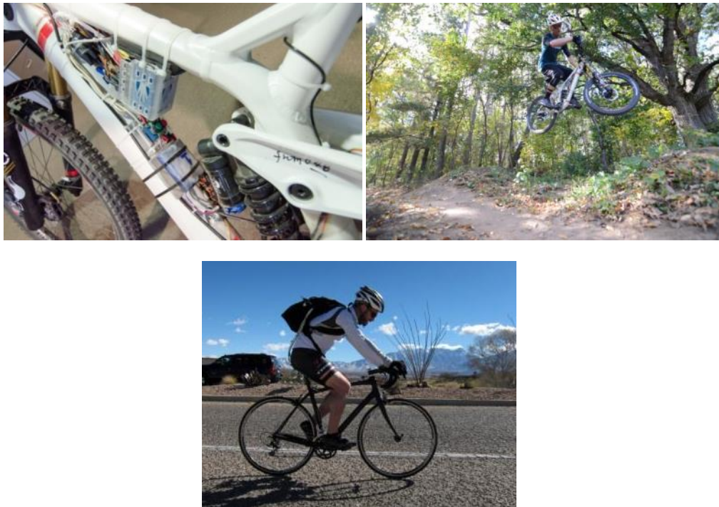
Figure 5. Session 29er mountain bike showing the DTS SLICE DAS (top). Old DAS requiring backpack and wire harness (bottom).
