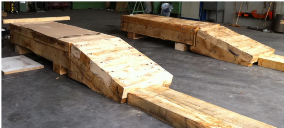
Figure 5 - Field Testing Setup to measure tread deformation
