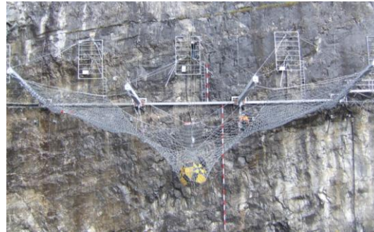
(c) 8000 kJ rockfall barrier test in Walenstadt
