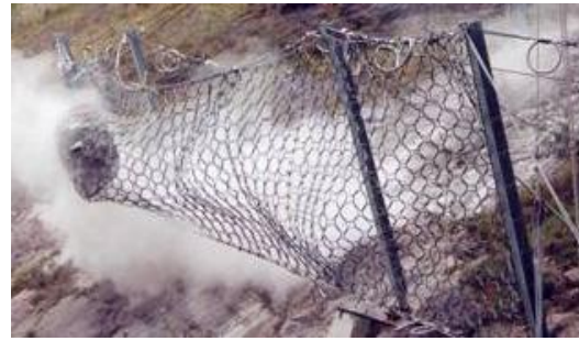
(b) Beckenried rockfall test
