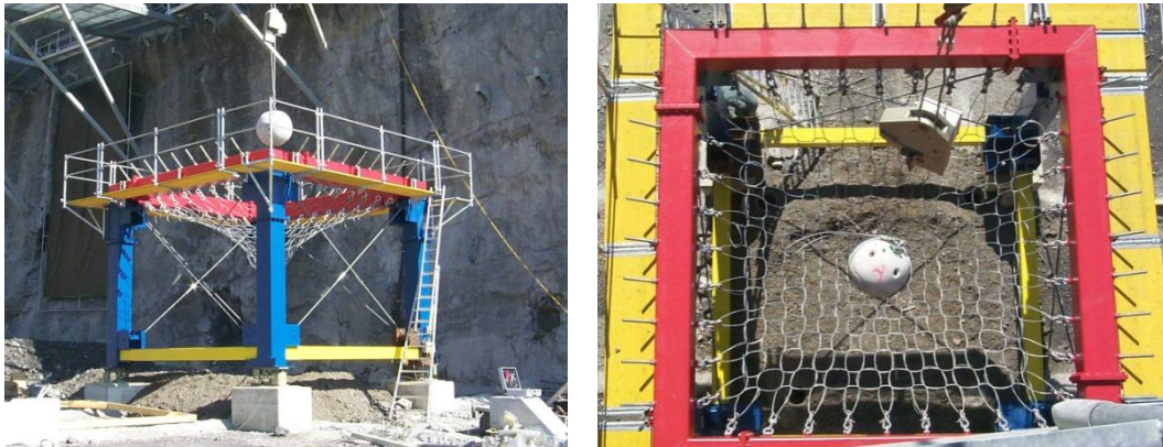
Figure 4. Test frame with a single spanned 16 m 2 square ring net with 5, 7, 12 and 19 windings per ring supported in a steel rigid frame: Boulder mass m = 825 kg, and falling heights from 3 m to 6 m (source: Grassl, 2002).
