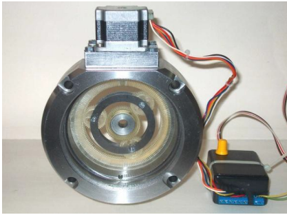
Fig. 3: Planetary gearbox driven by stepping motor
