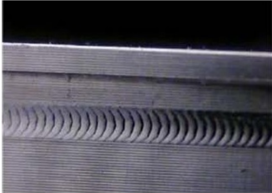
Figure 1. Typical laser welding pattern
