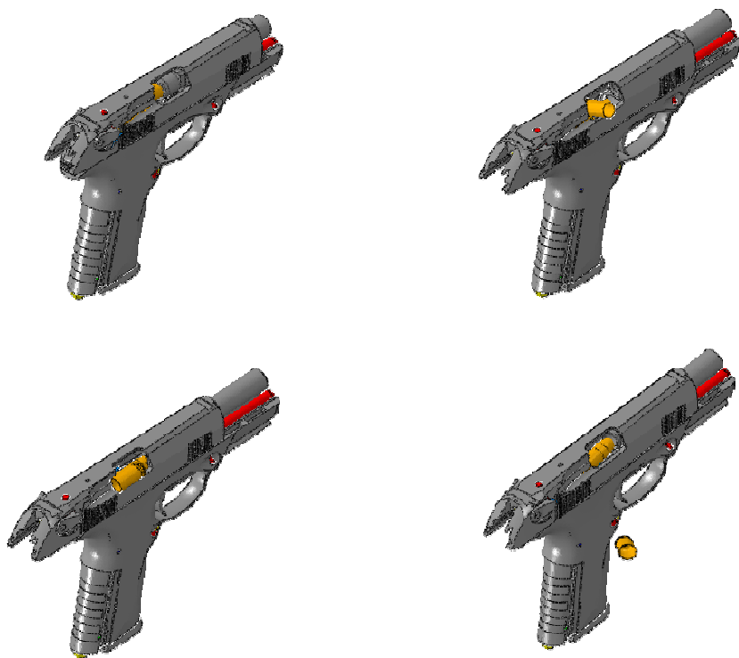
Figure 13. Deformed configurations at various times of the firing cycle.
