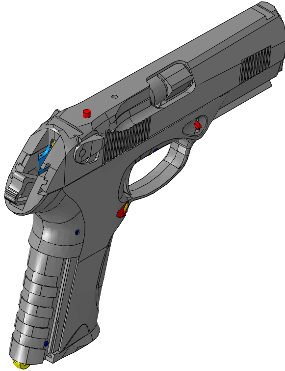
Figure 3. CAE model of the pistol with hammer cocked.
