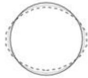
Figure 7. Initial (solid line) and deformed (dashed line) cross section of an elbow element.
