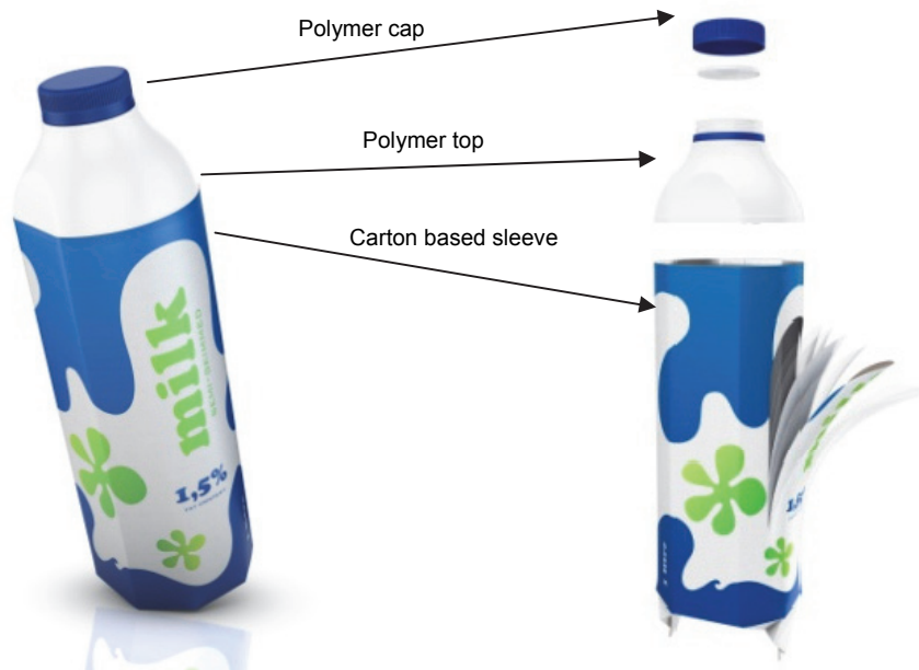
Figure 1. Tetra Evero Aseptic package with the different parts (Tetra Pak, 2012)
