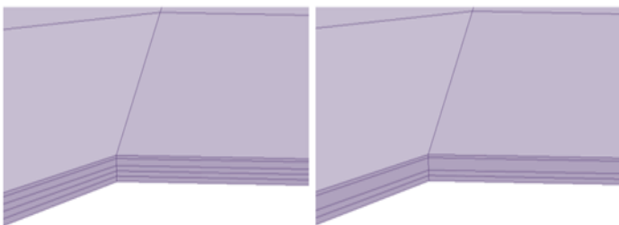
Figure 3: Zoomed views of the finite element mesh before editing (left) and after layers 2 and 3 from the top are merged (right).
