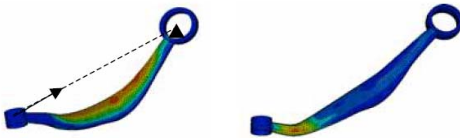
Figure 1. Comparison Between Linear Analysis(left) and Non- linear Analysis Results(right)
