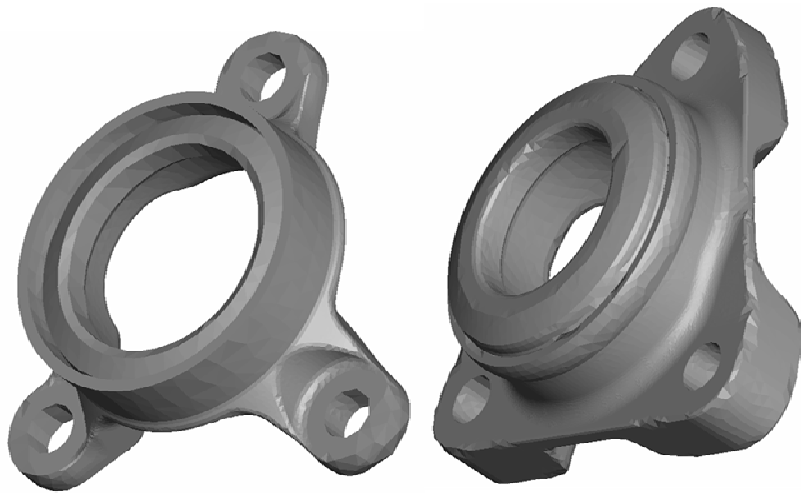
Figure 6. To the left: the original version of the forged piece, to the right: the modified reinforced version.
