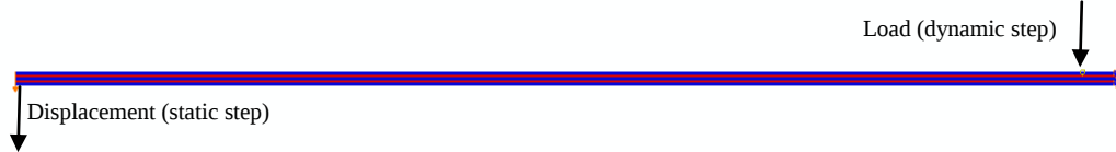
Figure 3. FE 2D planar model (cantilever beam).
