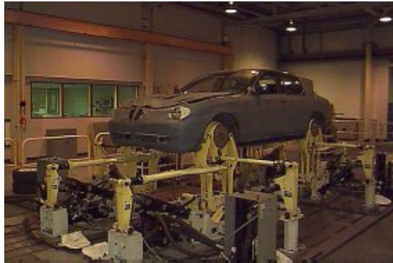
Figure 2: Multi-axis rig test showing time history load inputs at the wheel
