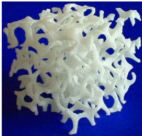
Figure 1. Scaled rapid-prototyping model of an auxetic foam sample [real dimensions: 0.1 x 0.1 x 0.1 mm].
