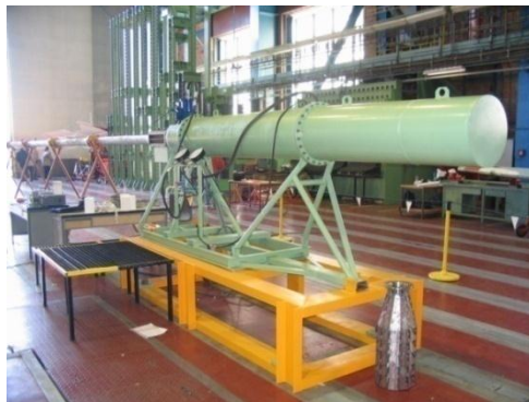
Figure 1. Air pressure tank, quick-opening valve, action and barrel body.
