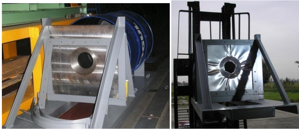
Figure 3. Arrangement for comparison between real and synthetic bird strike test.
