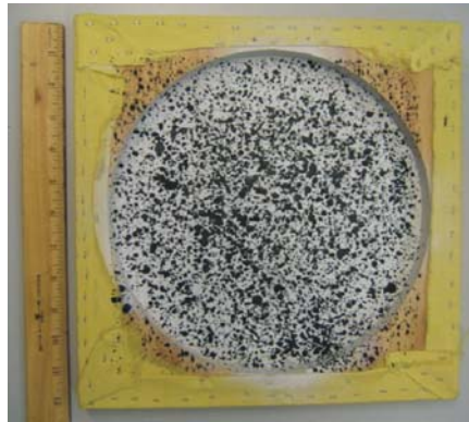
Figure 6. Back view (opposite side of impact) of Kevlar fabric specimen stapled to frame with R=12.7 cm round hole.
