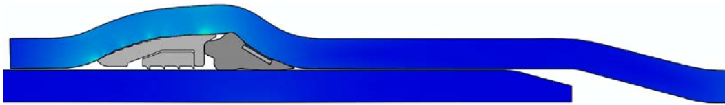
Figure 8. Pipe joint after assembly
