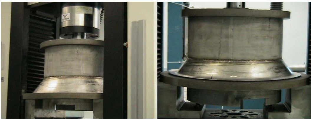
Figure 5 Experimental setup – left for pre-buckling and right for post-buckling.
