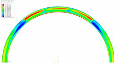
Figure 11: Repair Weld –Transverse Stress on Plane of Peak Stress –Moving Heat Source
