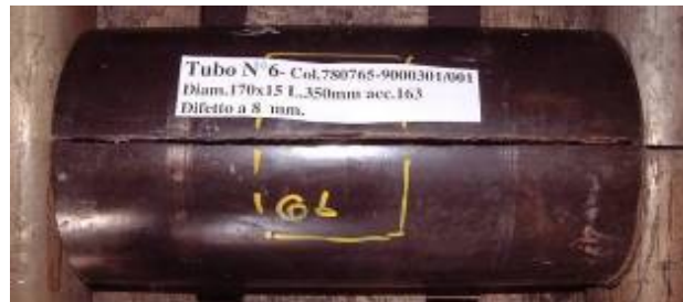
Figure 10 - Failure mode of a high toughness material (specimen #3)
