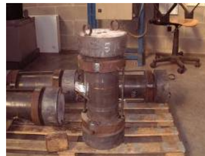
Figure 3 – a) Final crack depths and shape; b) Full scale specimens with caps used for the burst tests
