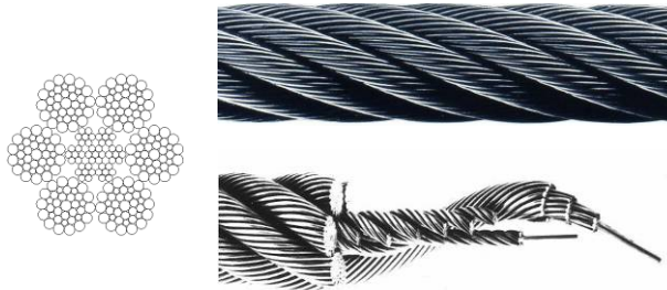
Figure 3: Stranded rope cross section and side view
