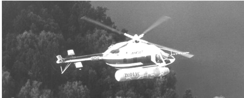
Figure 1. Helicopter with inflated ballonet
