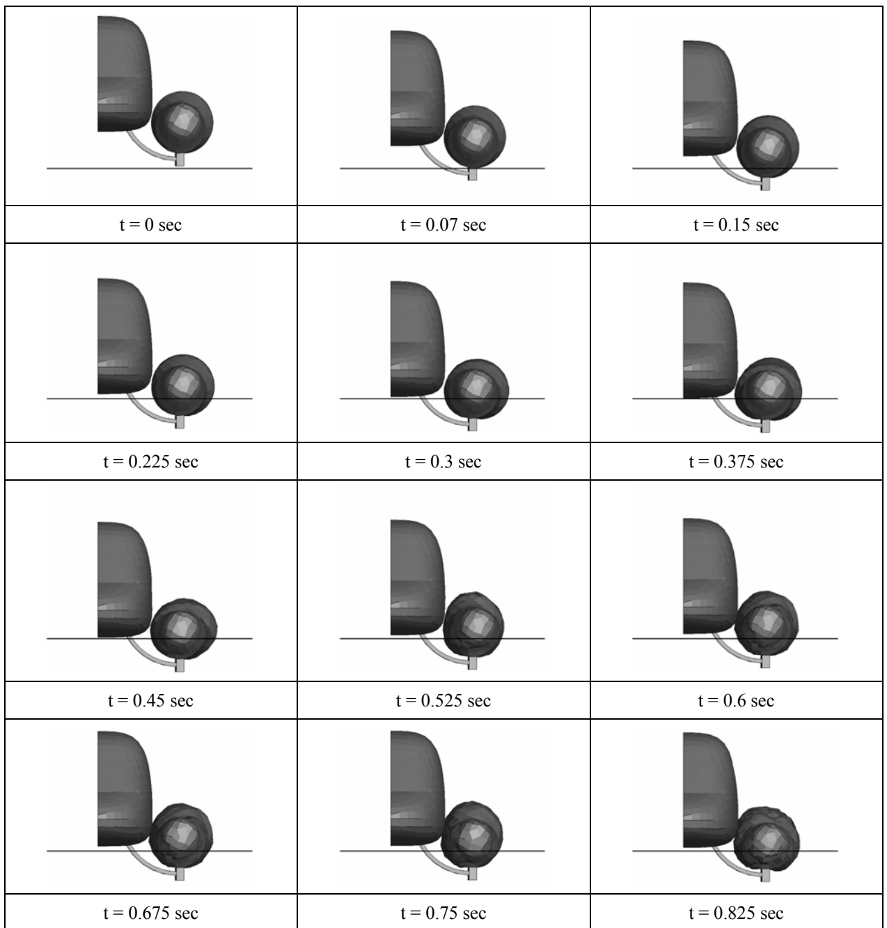
Figure 11 Deformation of ballonets at different times during splashdown of helicopter.
