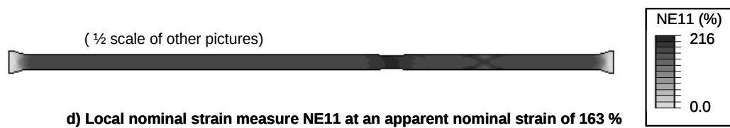
Figure 3: Depiction of local strain and stress measures as neck develops and propagates.
