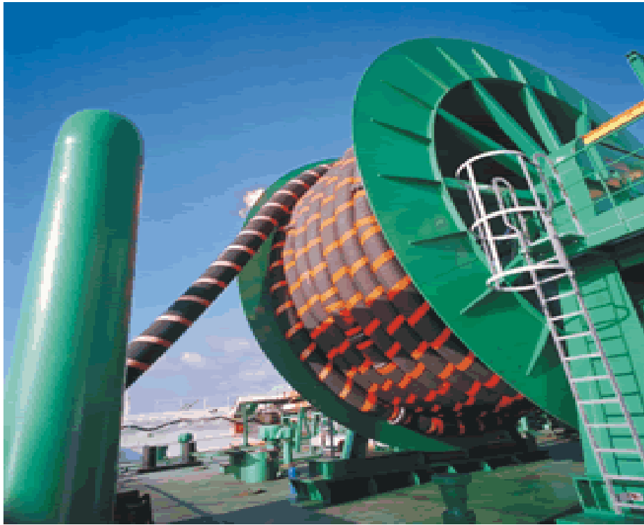
Figure2. Marine hose under the condition of reeling in the reel.
