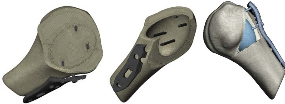
Figure 4. Showing the final mesh of the humerus, locking plate, cement and fractures
