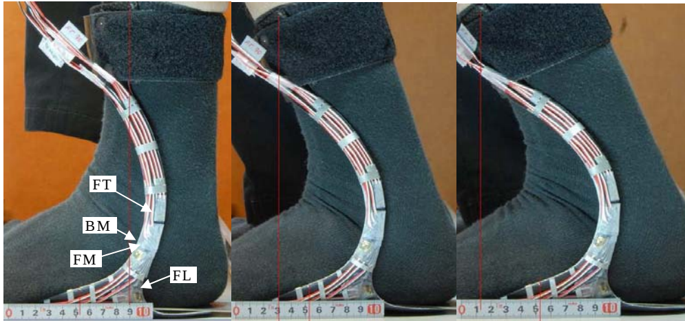
Figure 8. Full scale test: a) zero position, b) Horizontal deflected U = 58mm , c) Horizontal deflected U = 76mm
