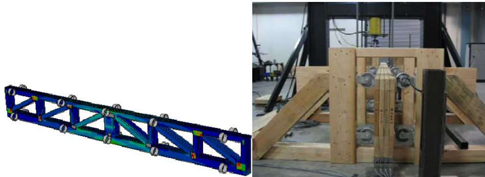
Figure 10. Four Ply Girder Truss Load Transfer Test
