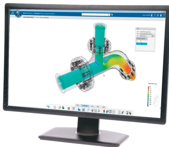
The Velocity Vector contour plot shows the direction of fluid flow in the simulation.
