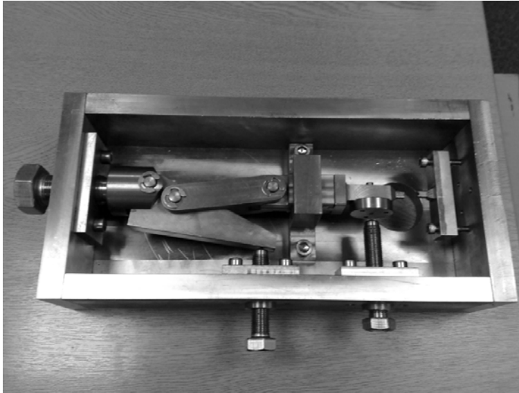
Figure 9. Loading device developed to perform compression and shear tests on a ruby and a polycrystalline alumina under a Raman microscope.
