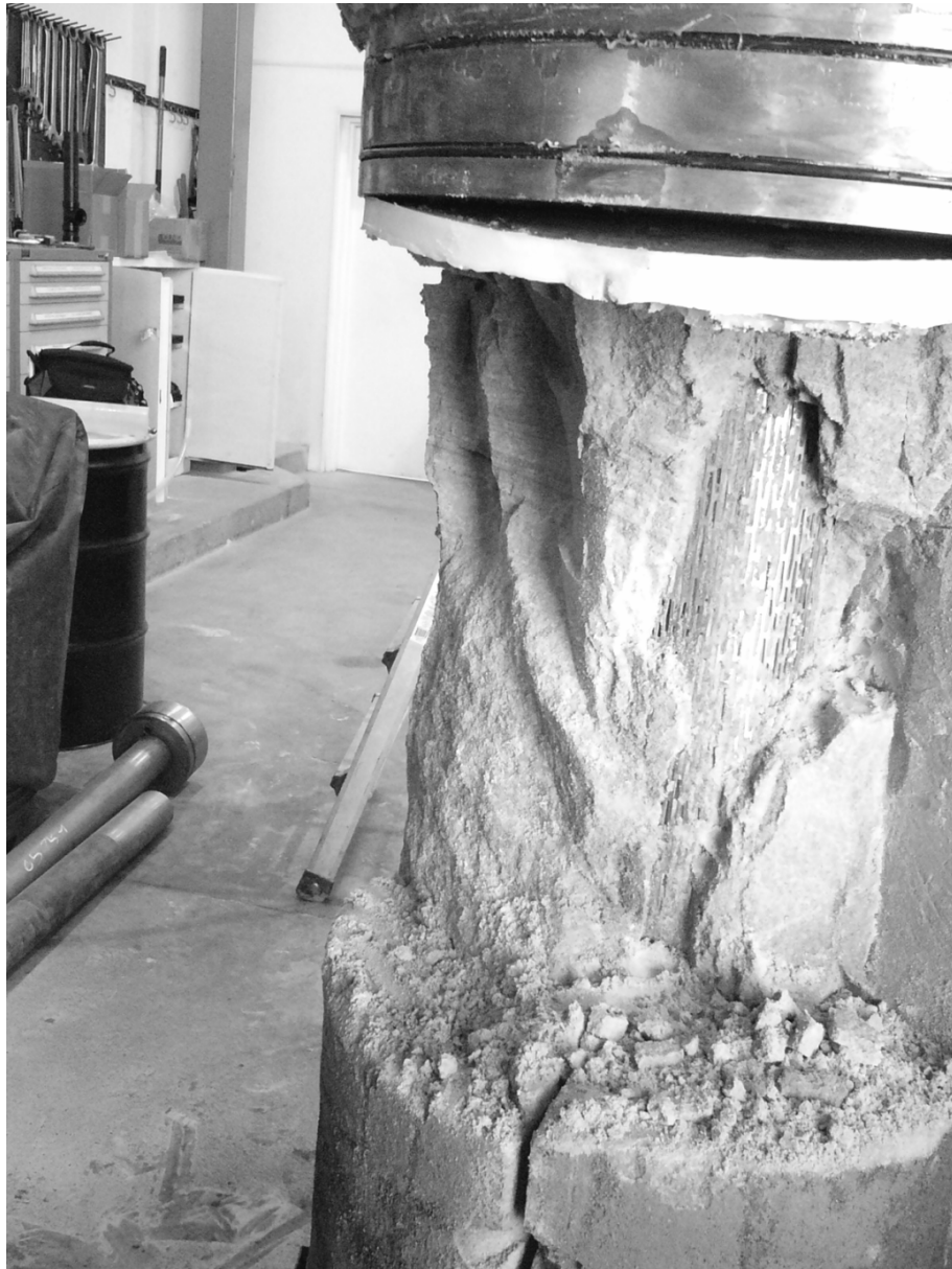
Figure 8 Partially dismantled rock sample showing ESS inside failed rock
