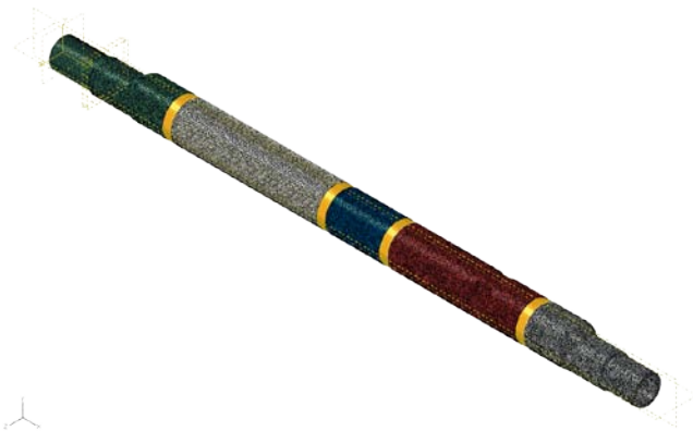
Figure 22. Meshed Side Pocket Mandrel with 2-in. welding parts
