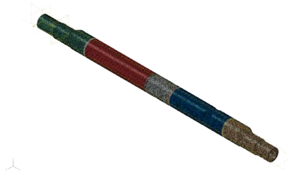
Figure 21. Meshed Side Pocket Mandrel with 1-in. welding parts
