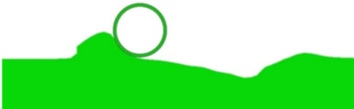
Figure 6: The pipe pushes the berm further laterally and has almost come out of the trench
