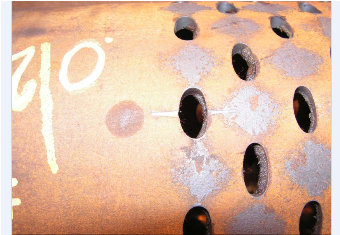
Figure 14 — A perforated basepipe with machined groove in the axial direction at the first row was expanded successfully at a rate 20% higher than current production rate.
