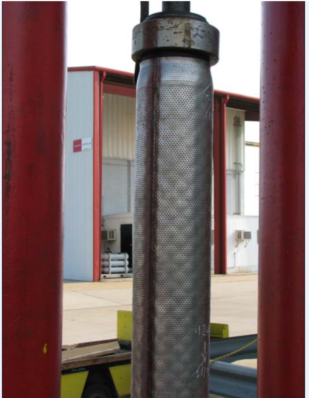
Figure 13 — A perforated basepipe with optimized hole pattern was expanded successfully at a rate 20% higher than current production rate.
