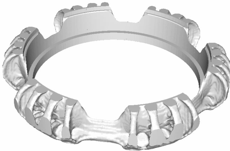
Figure 16. Optimized lens housing.
