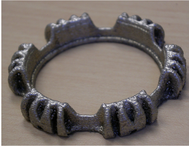
Figure 17. Prototype component manufactured from STL file.
