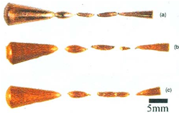
Figure 3. Dynamic Tensile Extrusion of Copper for grain size: (a) 65 \mu\text{m} , (b) 118 \mu\text{m} , (c) 185 \mu\text{m} .
