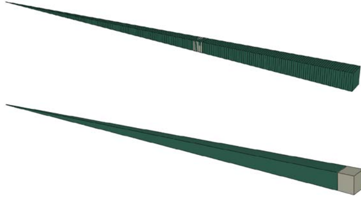
Figure 9. Hemispherical explosive CEL geometry, spherical symmetry.
