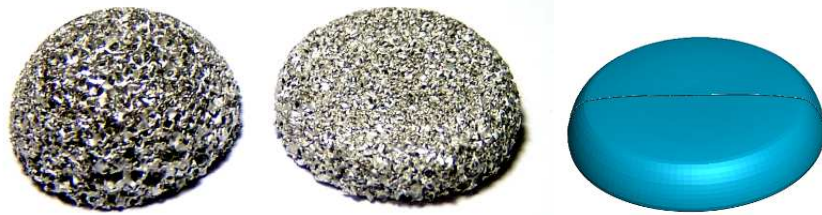
Figure 16. Comparison of model and experimental crush height – aluminum foam
