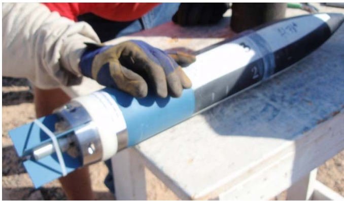
Photo of test projectile in carry to gun configuration
