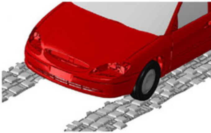
Figure 6: Vehicle on fatigue reference road (left), vertical acceleration of the right wheel center (right)
