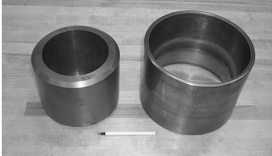
Figure 7 – Ring Rolling Process Steps for Creating a Double Race Cup
