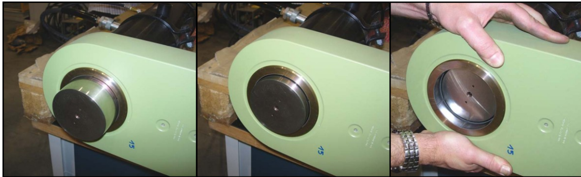
Fig. 4 –Cold expanded bushing installation process
