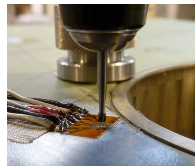
Fig. 12 - Hole-drilling tool and drilling operation
