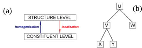
Figure 2. (a) Homogenization provides the ability to determine structure level properties from constituent level properties while localization provides the ability to determine constituent level responses from structure level results. (b) Example tree diagram.
