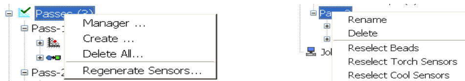
Figure 9. Sensor Options (a) regenerate sensors for the whole model (left) and (b) reselection of sensors (right) at pass level, if needed.
