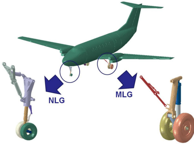
Fig. 1: Aircraft landing gear system
