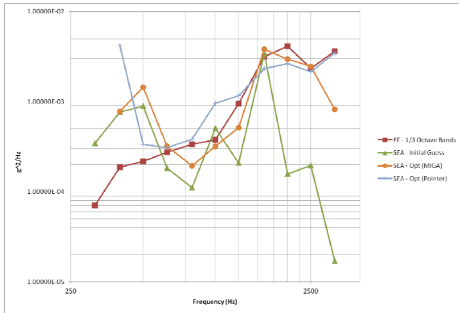
Figure 10. Comparison of ribbed panel vibroacoustic responses before and after optimization using Isight showing improved correlation.
