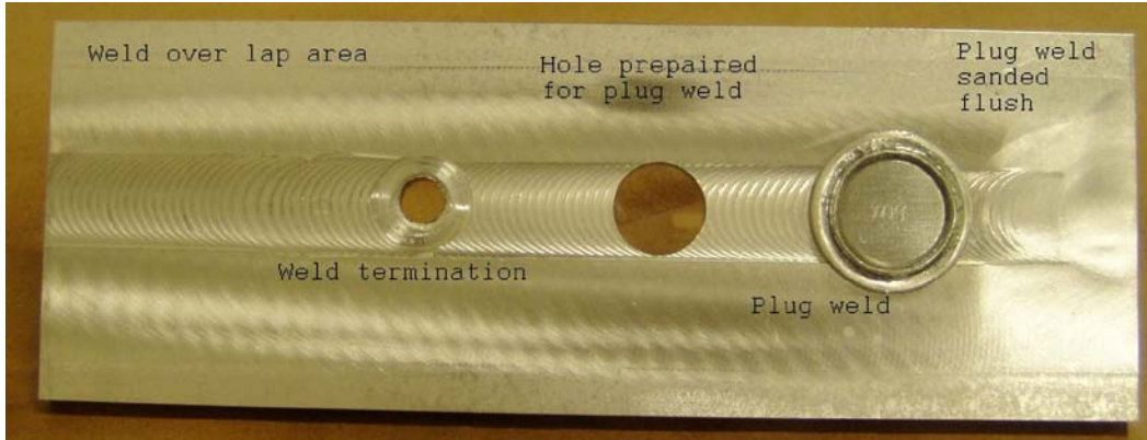
Figure 1. The test panel shows an example of a friction stir weld and a friction stir plug weld that fills the hole that is left when the stir weld tool is removed (NASA, 2008).
